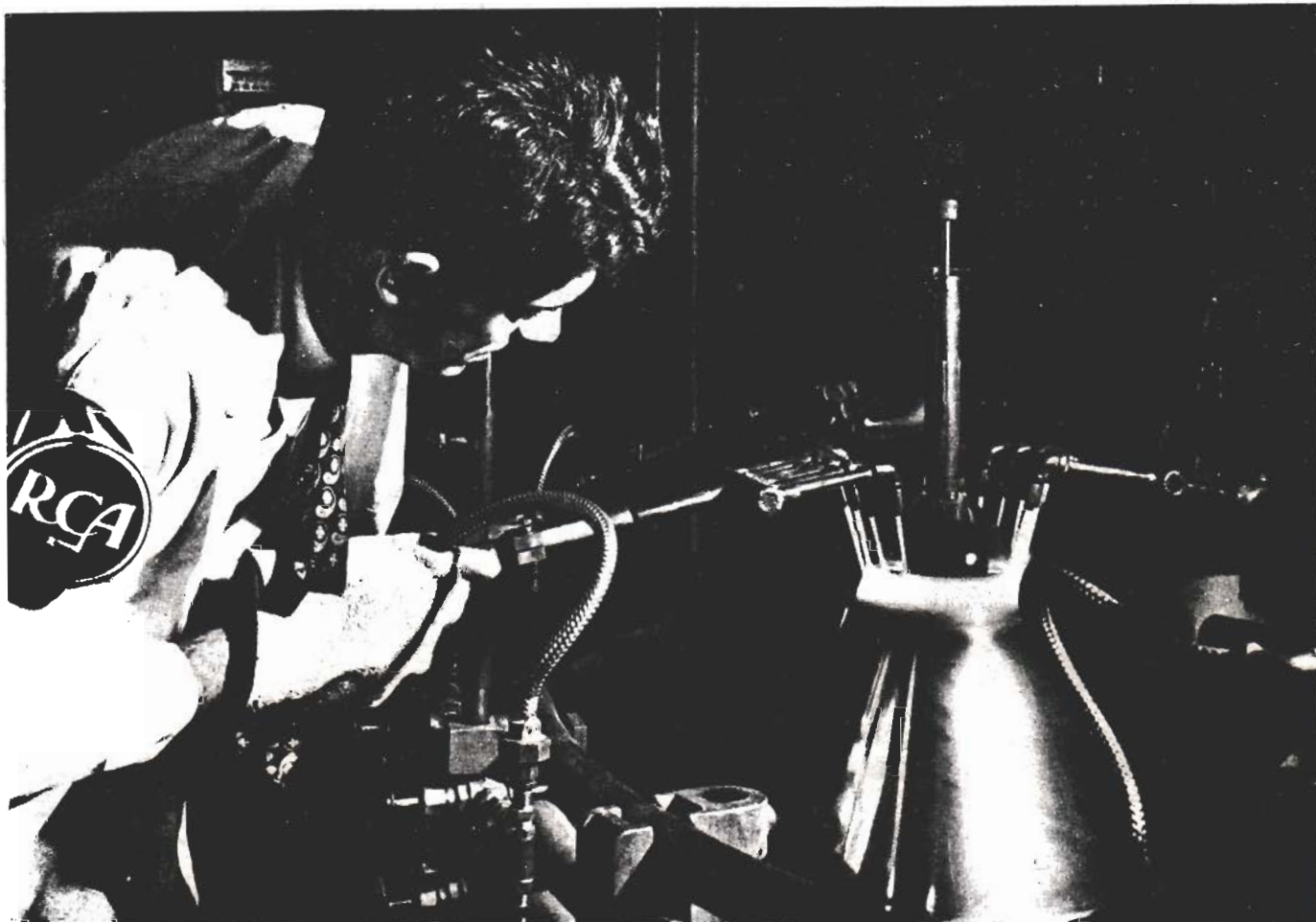
The glass neck section of a television picture tube is bonded to the metal cone on a high-speed production rotary machine employing Type "B" Oxygen-Gas Tips at the Lancaster Tube Plant of the Radio Corporation of America. As the machine indexes, glass and metal are sealed together in progressive steps from preheating to final annealing.
